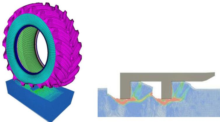
Examples of SPH simulation applied to soft soil
